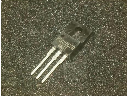
Fig. 2: The PGA26C09DV [25] HD-GIT sample in TO-220D package
